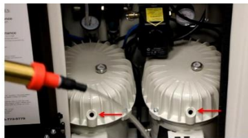
Pour New Oil Through The Compressor Pump Intake Holes
