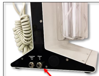
Filtered Air in female quick disconnect fitting on Table-Top model
