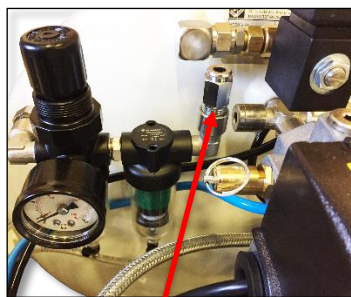
Compressor Regulator In-Line female quick disconnect fitting
