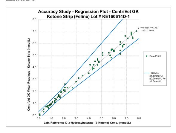
N = 120Slope = 0.8855 Intercept = 0.1367  $R^2 = 0.9893$  CentriVet Blood Glucose and Ketone Meter Reading – CentriVet Blood Ketone Strip vs. Laboratory Reference Method, Feline Whole Blood Sample: All 3 Strip Lots KE160518C-1, KE160614C-1, and KE160614D-1 Combined
