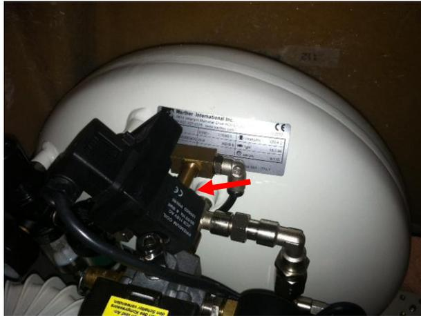
**11. Secure the Auto Drain control module box to the brass bar using the silver hex nut.**
