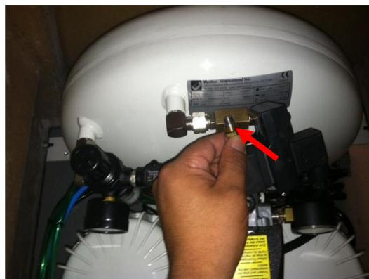
**10. Slide the Auto Drain control module box back onto the brass bar.**
