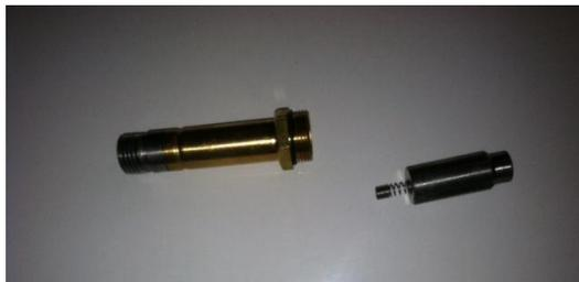
6. Remove any debris or build up and use rubbing alcohol to clean inside the Auto Drain valve.
