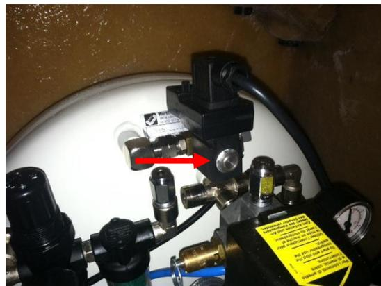
**12. Connect the compressor/unit to an electrical outlet to test it. Press the test button on the top of the Auto Drain control module box to test the Auto Drain. You should hear a burst of air; this is the Auto Drain purging the compressor holding tank into the collection bottle, meaning the Auto Drain is functioning properly.**
