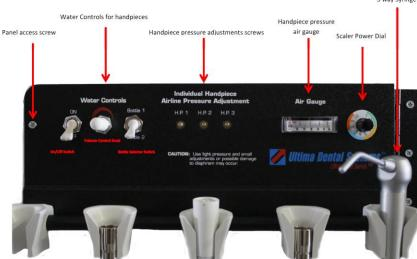
3. Once you have access to the air gauge, remove the two silver hex nuts on either side.
